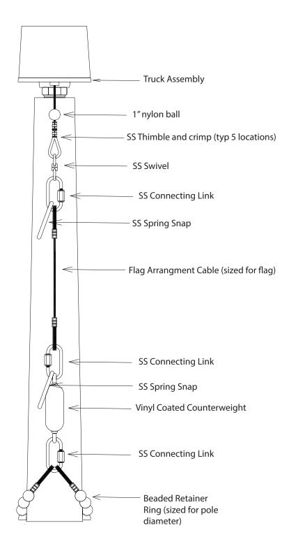
1) For flags of 15'x25' and larger add shock spring between swivel and upper SS connecting link
