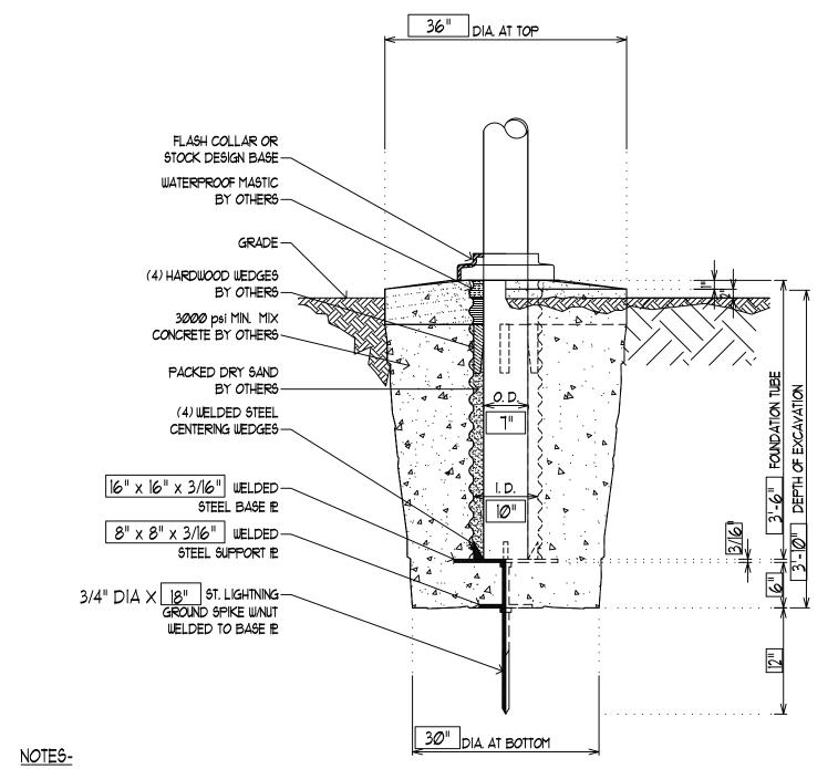
THIS FOUNDATION DETAIL IS A RECOMMENDATION ONLY AND IS BASED ON GOOD, FIRM, DRY SOIL. ACTUAL FOUNDATION DESIGN IS THE RESPONSIBILITY OF THE PROJECT ENGINEER. IF ADDITIONAL FOUNDATION DEPTH IS REQUIRED, THE SPIKE CAN BE LENGTHENED AND THE DISTANCE BETWEEN THE BASEPLATE AND SUPPORT PLATE CAN BE INCREASED.
